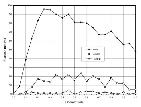
**Figure 1.** Comparison of inversion (Inver), gene deletion/insertion (Del/Ins), and restricted permutation (Permut) on the traveling salesperson problem with 19 cities. For this analysis P = 100 and G = 200. The success rate was evaluated over 100 identical runs.
